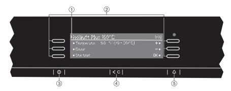
The appliance is operated via the display ① and the electronic sensors next to and below the display. These react to finger contact. A keypad tone will sound each time a sensor is touched. The volume of the keypad tone can be adjusted or switched off altogether (see "Settings - Volume - Keypad tone").
